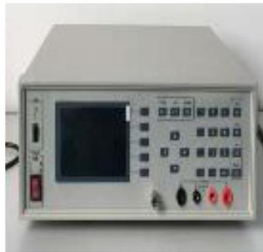
**FT-300A Resistance Testing Instrument**
